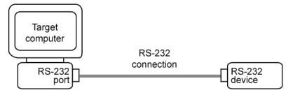
Your real-time applications can use these RS-232 ports as I/O devices. With the typical DTE/DCE configuration of the RS-232 device, the target computer is connected to the device with a null modem cable.
