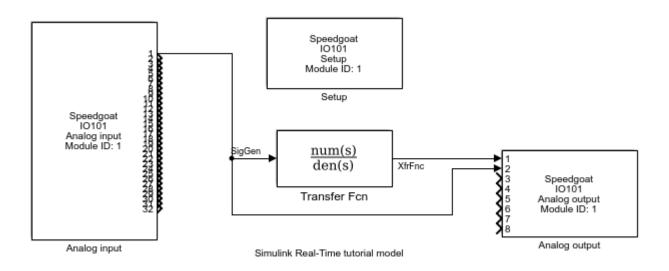
You cannot run this model unless the required I/O board is installed in your target computer. You can substitute driver blocks for another I/O board that is installed in the target computer.
