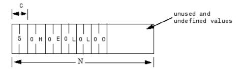
The serial blocks interpret each entry in the vector as a single character. The low-level Send block writes the low-order byte of each entry to the UART. The 16-bit and 32-bit data types allow the embedding of 8-bit data values, including 0. The 8-bit data type is most useful with the ASCII Encode and Decode blocks. The 16-bit and 32-bit data types are most useful for binary data streams.
