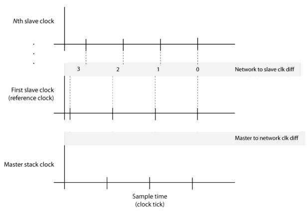
In phase 2, the algorithm shifts the sample time of the master stack running on the target computer to align with the first slave node clock. In that process, the EtherCAT Init block output value MasterToNetworkClkDiff decreases to near zero. If there are no DC enabled devices, both values are zero.
