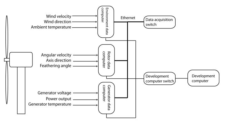
To record the data and timestamps, connect the sensors to a set of data acquisition target computers. Interconnect the data acquisition computers through an Ethernet network and a switch that supports the PTP protocol (a PTP transparent clock or boundary clock). To access the data and timestamps, connect the target computers to a development computer through another Ethernet network and switch. On the development computer, run MATLAB to do the data analysis, including:
