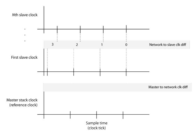
In phase 2, the algorithm shifts the sample time of the first DC-enabled slave node to align with the clock of the master stack. In that process, the value MasterToNetworkClkDiff decreases to near zero. The algorithm shifts the sample time of the other network nodes to stay aligned with the first slave node clock. In that process, the value of NetworkToSlaveClkDiff can first increase, then decrease to near zero.
